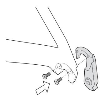
Apply Loctite 242 to the fixing screws, and tighten the screws equally to a maximum of 1 Nm.
