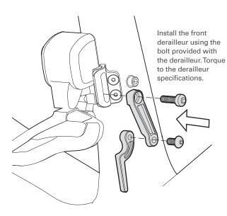
Install chain catcher when installing the front derailleur. Complete final adjustment with the chain in the small chainring and largest cassette cog. Tighten the connecting bolt to 4 Nm.
