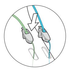
Install cable housing (with ferrules) into individual Mechanical Brake & Shifter Cable Stop until the housing rests securely in the pockets. Route cables to bottom bracket, ensuring they are not twisted together.
