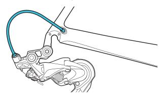
As per manufacturer's instructions, install rear derailleur on rear derailleur hanger, cut appropriate housing length, and attach cable.
