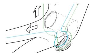
The front cable travels across the non-drive side slot, and in the direction of the seat tube. The rear cable travels along the drive side slot, and along the chain stay. When complete, snap Bottom Bracket Cable Guide into place.
